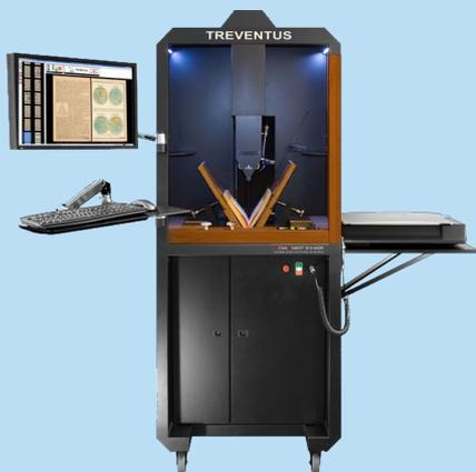
We have deployed two Treventus ScanRobot® 2.0 which are high speed mass digitisation systems (MDS) designed for large volume digitisation of any bound material.
